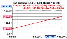
The range between RoHS and RoLS should be over 20% of span at least; otherwise, it will be got less resolution of analogue output.
