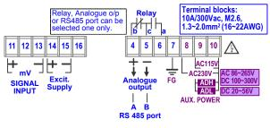
Please check the voltage of power supplied first, and then connect to the specified terminals. It is recommended that power supplied to the meter be protected by a fuse or circuit breaker.
