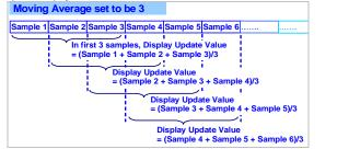
Remark: The higher moving average setting wouldn't cause the response time of Relay and Analogue output slower after first 3 samples.
