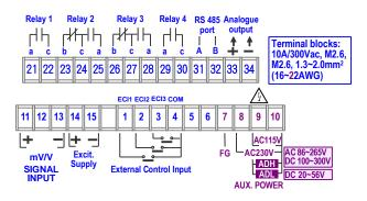
Please check the voltage of power supplied first, and then connect to the specified terminals. It is recommended that power supplied to the meter be protected by a fuse or circuit breaker. **Power Supply**
