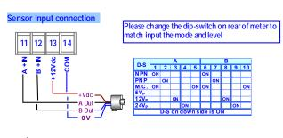
Connected to 11 (A + IN), 12 (B + IN) pin signal level required toclear the high and low potential.
