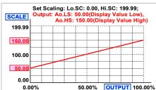
The range between RoH5 and RoL5 should be over 20% of span at least; otherwise, it will be got less resolution of analogue output.
