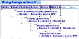
Remark: The higher moving average setting wouldn't cause the response time of Relay and Analogue output slower after first 3 samples.
