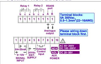
Please check the voltage of power supplied first, and then connect to the specified terminals. It is recommended that power supplied to the meter be protected by a fuse or circuit breaker.
