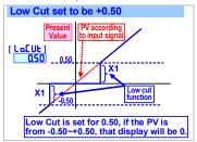
If set the negative value (X2) here to display "X2" which it expressed to be low-cut the PV that it's under the X2 setting value:
