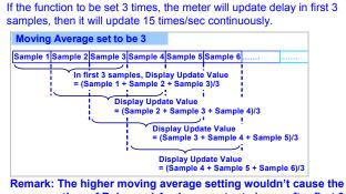
response time of Relay and Analogue output slower after first 3 samples. The digital filter can reduce the magnetic noise in field.
