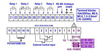
Please check the voltage of power supplied first, and then connect to the specified terminals. It is recommended that power supplied to the meter be protected by a fuse or circuit breaker.
